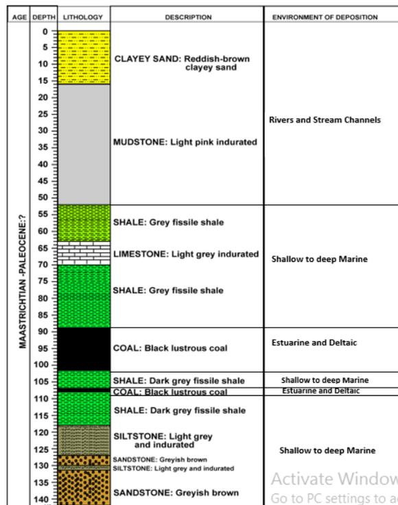
Figure 4. Litho-section showing Araromi Well.
