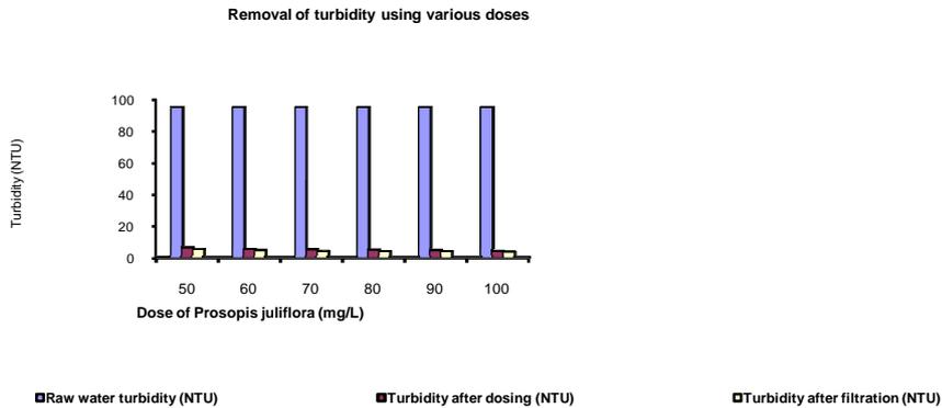
Figure 2. Removal of turbidity using various doses of *Prosopis juliflora* (for highly turbid water).
