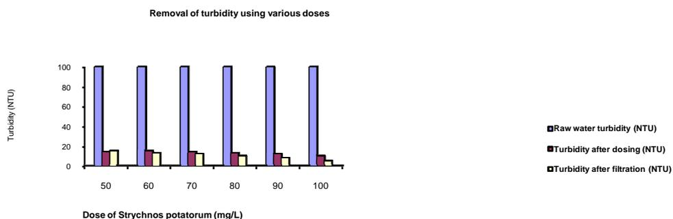
Figure 1. Removal of turbidity using various doses of *Strychnos potatorum* (for highly turbid water).
