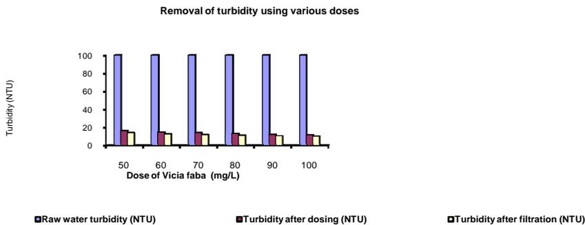
Figure 3. Removal of turbidity using various doses of *Vicia faba* (for highly turbid water).
