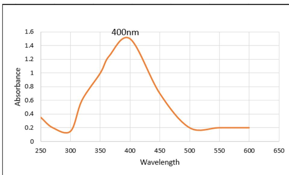
**Figure 14. UV-Vis absorption spectra of 4-nitrophenol taken after addition of  $\text{NaBH}_4$ .**
