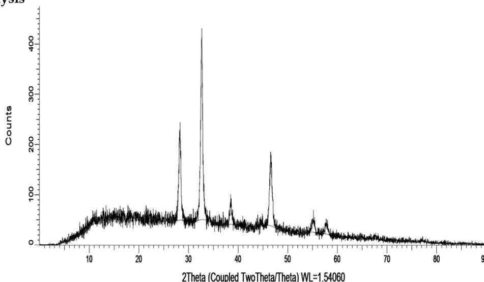
Figure 8. XRD pattern of biosynthesized silver nanoparticles.
