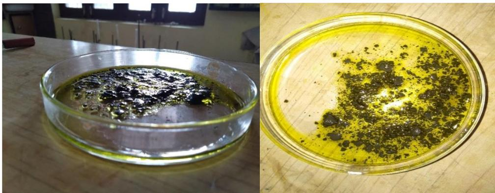
Figure 1. Silver Nano particles dipped in acetone in a Petri dish.
