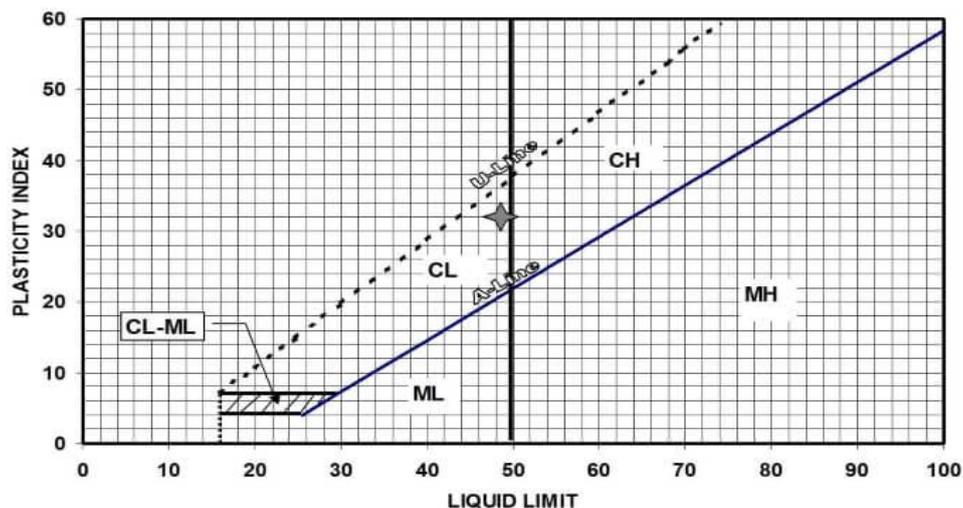
**Figure 5. Plasticity andix for soil classification.**
